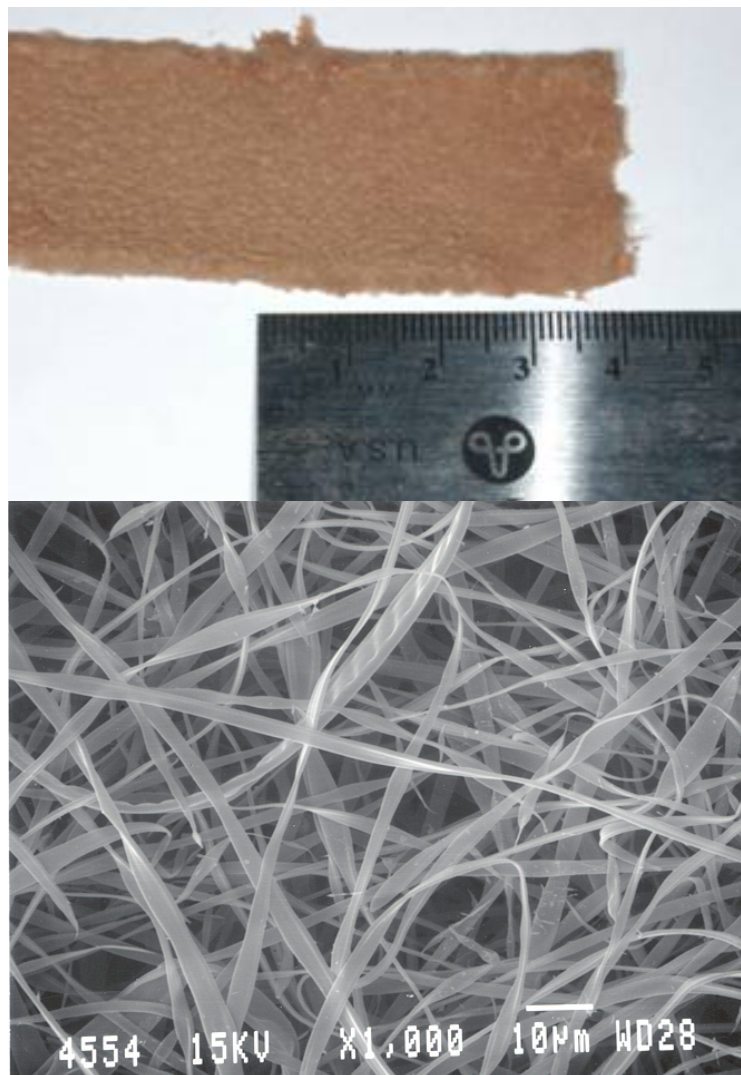
Figure 3.3. Photograph (top) and scanning electron micrograph (bottom) of a hemoglobin scaffold electrospun from a 175 mg/ml solution.
